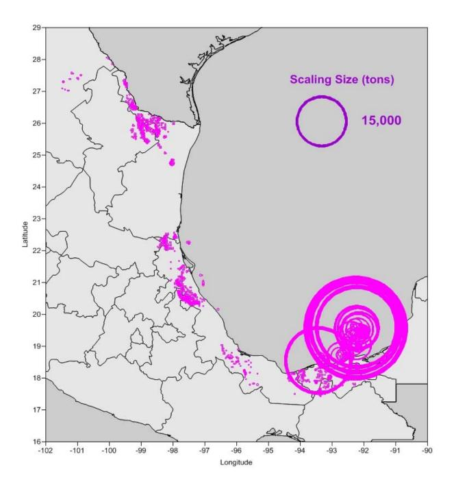
**Figure 15.** Annual 2016 SO<sub>2</sub> emissions (individual wells aggregated to 4km by 4km grid cells). Location symbols are proportionally sized by emissions.
