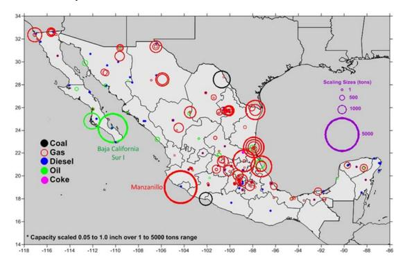
**Figure 28.** SO<sub>2</sub> emissions (tons) from thermal electricity generation during 2016; location symbols are sized by emissions.
