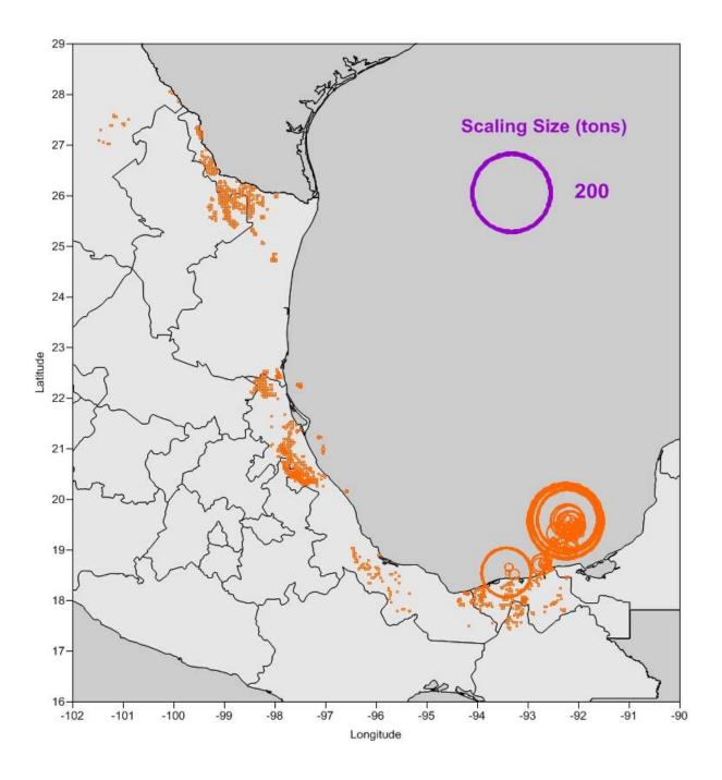
**Figure 16.** Annual 2016 PM<sub>2.5</sub> emissions (individual wells aggregated to 4km by 4km grid cells). Location symbols are proportionally sized by emissions.
