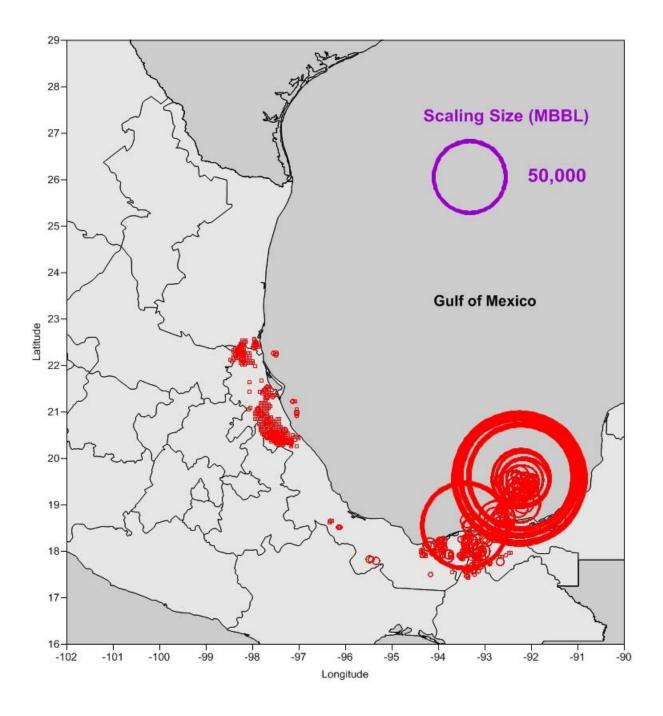
**Figure 5.** Annual 2016 natural gas production (individual wells aggregated to 4km by 4km grid cells). Location symbols are proportionally sized by production (MMcf).
