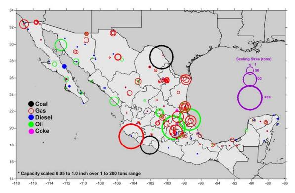
**Figure 30.** PM<sub>2.5</sub> emissions (tons) from thermal electricity generation during 2016; location symbols are by emissions.
