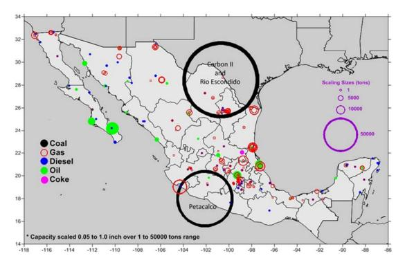
**Figure 27.** CO emissions (tons) from thermal electricity generation during 2016; location symbols are sized by emissions.
