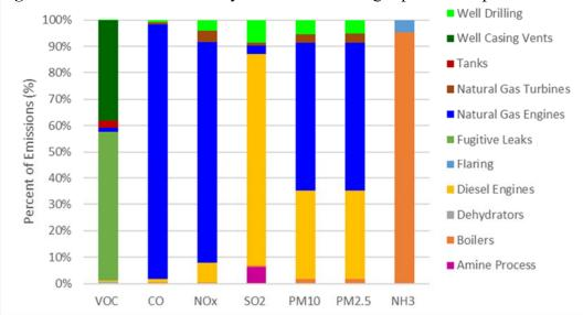
Figure 7. Percent of emissions by SCC from oil and gas production platforms\*.
