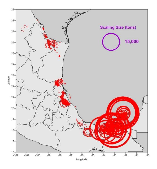
**Figure 14.** Annual 2016 CO emissions (individual wells aggregated to 4km by 4km grid cells). Location symbols are proportionally sized by emissions.
